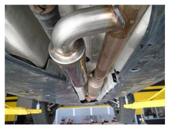
**Step 2:** Begin Installing the new MagnaFlow system by attaching the Resonator Assembly to the OE outlet using the OE fasteners and supplied gasket.
