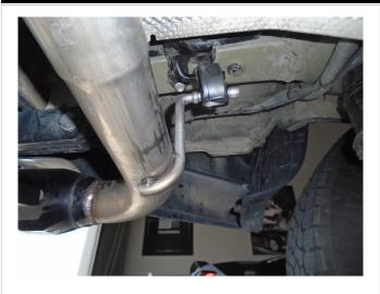
Finish the installation by fitting the Tail Pipe Assemblies onto the Muffler Assembly using the supplied clamps and fitting the hangers into the rubber insulators.
