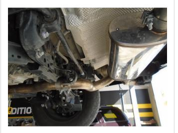
**Step 3:** Next, attach the Muffler Assembly to the Resonator using the supplied 2.50 Clamp and by fitting the hanger into the rubber insulator.
